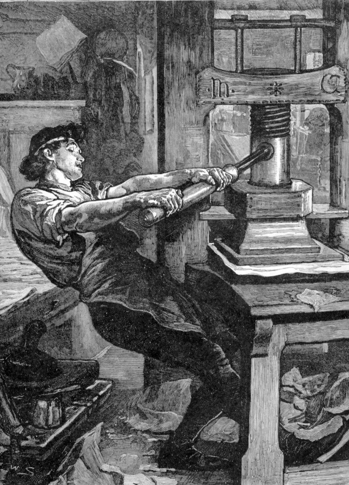
A black and white engraving of a man operating a large printing press. He is wearing a cap and a dark shirt, and is pulling on a long, thick lever or handle that extends from the side of the press. The press itself is a large wooden structure with various mechanical parts, including a large cylinder and a screw mechanism. The background shows a workshop environment with shelves and other equipment.
